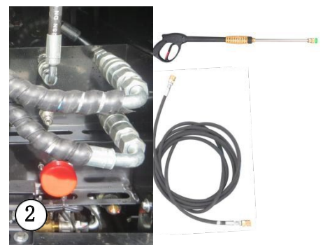
High pressure water quick connection
