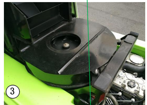
Clean the turbine fan through this opening
