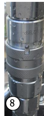
Rotary Retaining Ring, Lock the Hydraulic Quick-Connect Fitting
