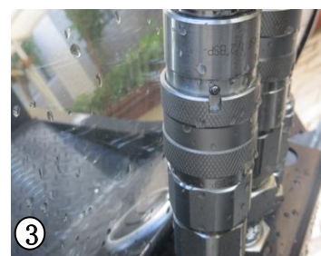
Rotary Retaining Ring, lock the Hydraulic Quick-Connect Fitting
