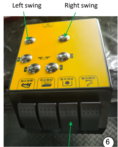
Fan pump button (press up for fan and spray water, press down only for fan)
