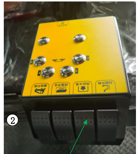
Turbine Fan + Spraying Switch ( Pressing upwards activates both the fan and spraying function, Pressing down activates the fan only)
